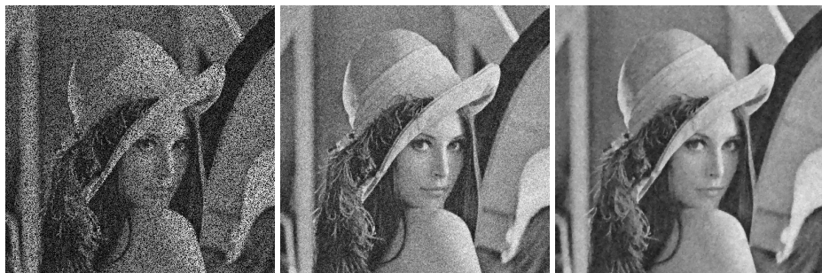
(a) Corrupted image MR = 30%, \sigma = 40 (b) Pre-completion result (c) TV PSNR = 28.27dB
