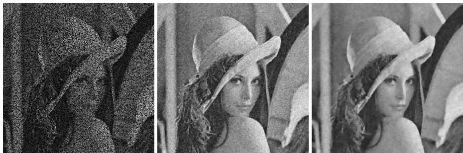
(a) Corrupted Image MR = 50%, \sigma = 40 (b) Pre-completion result (c) TV PSNR = 26.95dB
