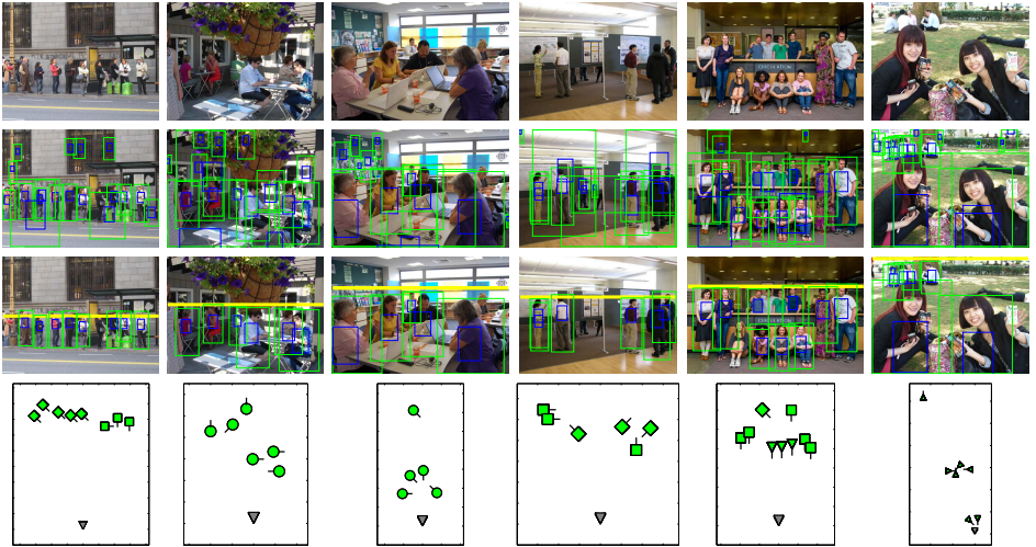
Fig. 5: Example results of our 3D estimation. The first row shows the input image. The second row shows the input Poselet detection [1]. The full body bounding boxes are colored green and the torso bounding boxes are colored blue. Note that the input detections are often noisy, e.g. bad localization and truncation by the image. The third row shows the horizontal line (yellow) and the true positives returned by our method. Our method is able to remove false positives. The last row shows the 3D map in a top-down view. Squares represent standing people, circles represent people sitting on an object, and triangles represent people sitting on the ground. The view point of each individual is shown with a line. The gray triangle is the camera position. This shows our method’s ability to generate 3D estimates which are robust to noisy 2D bounding boxes.
