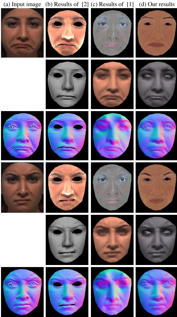
Fig. 3. Comparison of intrinsic images and 3D shapes. (a) Input images and ground-truth geometry. (b) Results of [2]. (c) Results of SIRFS [1]. (d) Our results. For each example, the first row is reflectance, the second row is shading, and the last row is a normal map.
