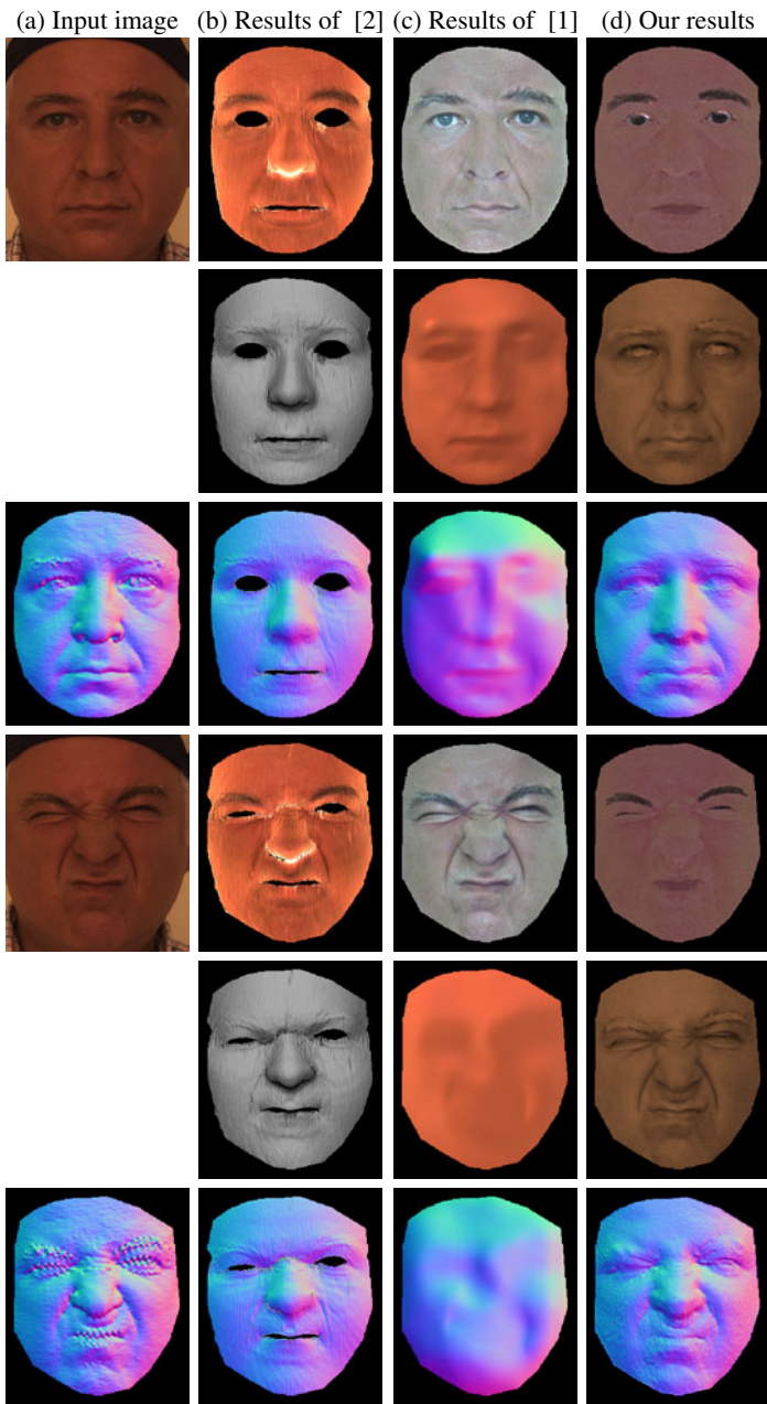
Fig. 8. Comparison of intrinsic images and 3D shapes. (a) Input images and ground-truth geometry. (b) Results of [2]. (c) Results of SIRFS [1]. (d) Our results. For each example, the first row is reflectance, the second row is shading, and the last row is a normal map.
