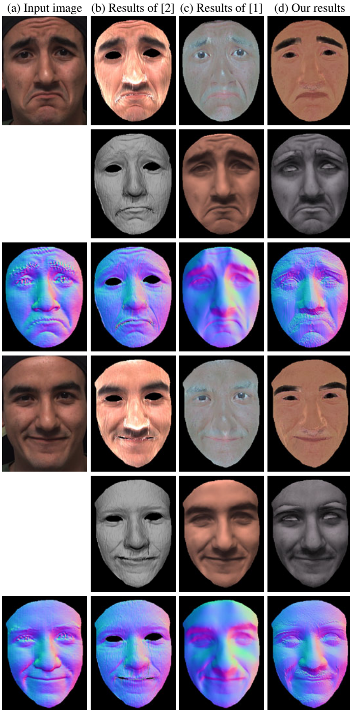
Fig. 5. Comparison of intrinsic images and 3D shapes. (a) Input images and ground-truth geometry. (b) Results of [2]. (c) Results of SIRFS [1]. (d) Our results. For each example, the first row is reflectance, the second row is shading, and the last row is a normal map.
