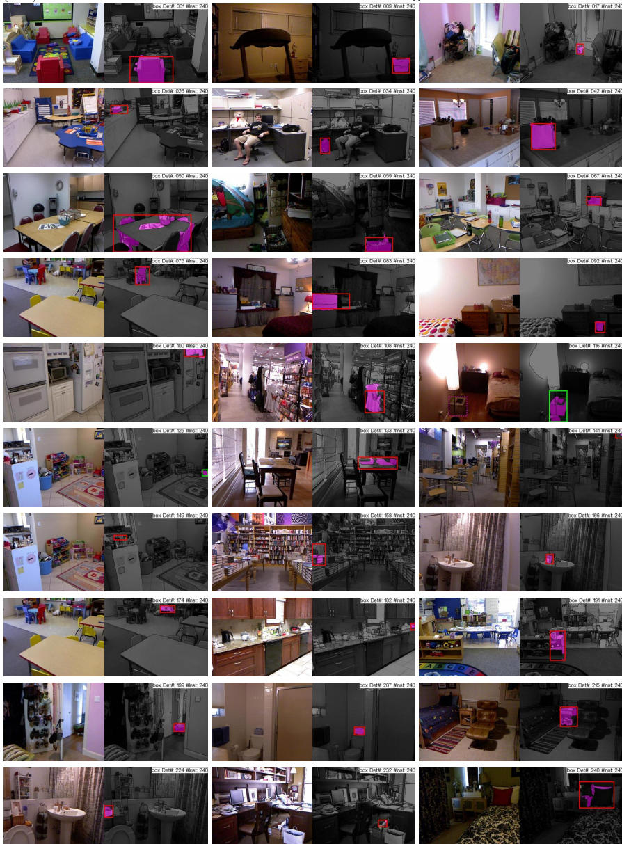
Fig. 19. Output of our box detector: We visualize 30 detections uniformly sampled from the first numInsts detections. The examples are laid out row-wise with 3 examples per row. The first image has the ground truth bounding box and the second image shows the output from the object detector color coded as follows: true positive (green), duplicate detection (blue), mis-localization (yellow) and confusion with other categories (red). We also mark the mask for each detection in magenta.
