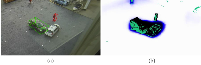
Fig. 4. Simultaneously detecting people and cars. (a) A person and a car is detected, as indicated by the red and green wireframes. (b) The same boxes are projected and filled as black boxes to create a synthetic image that approximates as closely as possible the background subtraction results, shown in green. Note that the white car is the same as the one that appears in Fig. 1. It remains undetected because the background subtraction algorithm fails to extract it.
