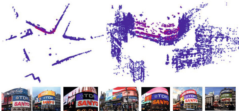
Fig. 6. Identification of dynamic textures within existing SfM estimates. Top Row: birds-eye and frontal view of estimated sparse structure for Piccadilly Circus. Blue dots are 3D features with persistent color across the dataset. Red dots are 3D features determined to have sporadic color. The bottom row shows sample images in the dataset. We associate color persistence with predominantly linear variation in the RGB space.
