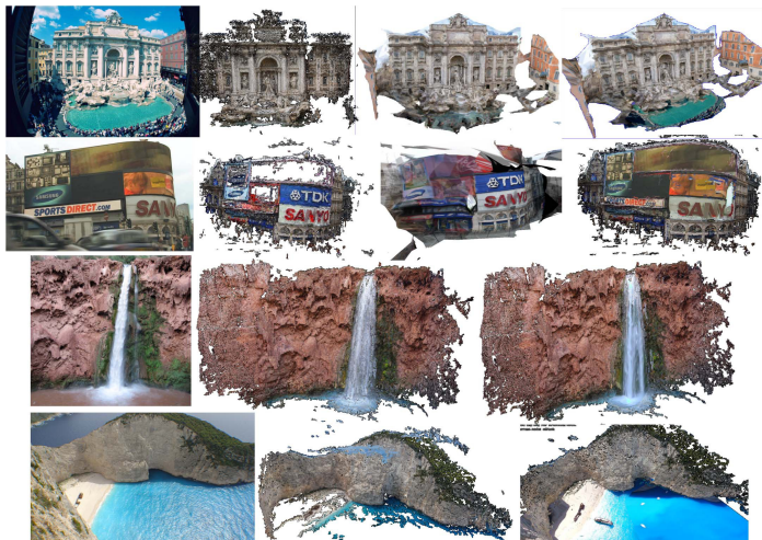
Fig. 9. Top two rows: sample dataset imagery, respective outputs for PMVS, CMPMVS and our proposal. Bottom two rows: sample dataset imagery, respective outputs for PMVS and our proposal; CMPMVS failed to generate on the same input data.
