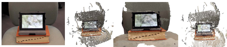
Fig. 10. From left to right: sample dataset imagery, respective outputs of PMVS, CMPMVS and our proposed method
