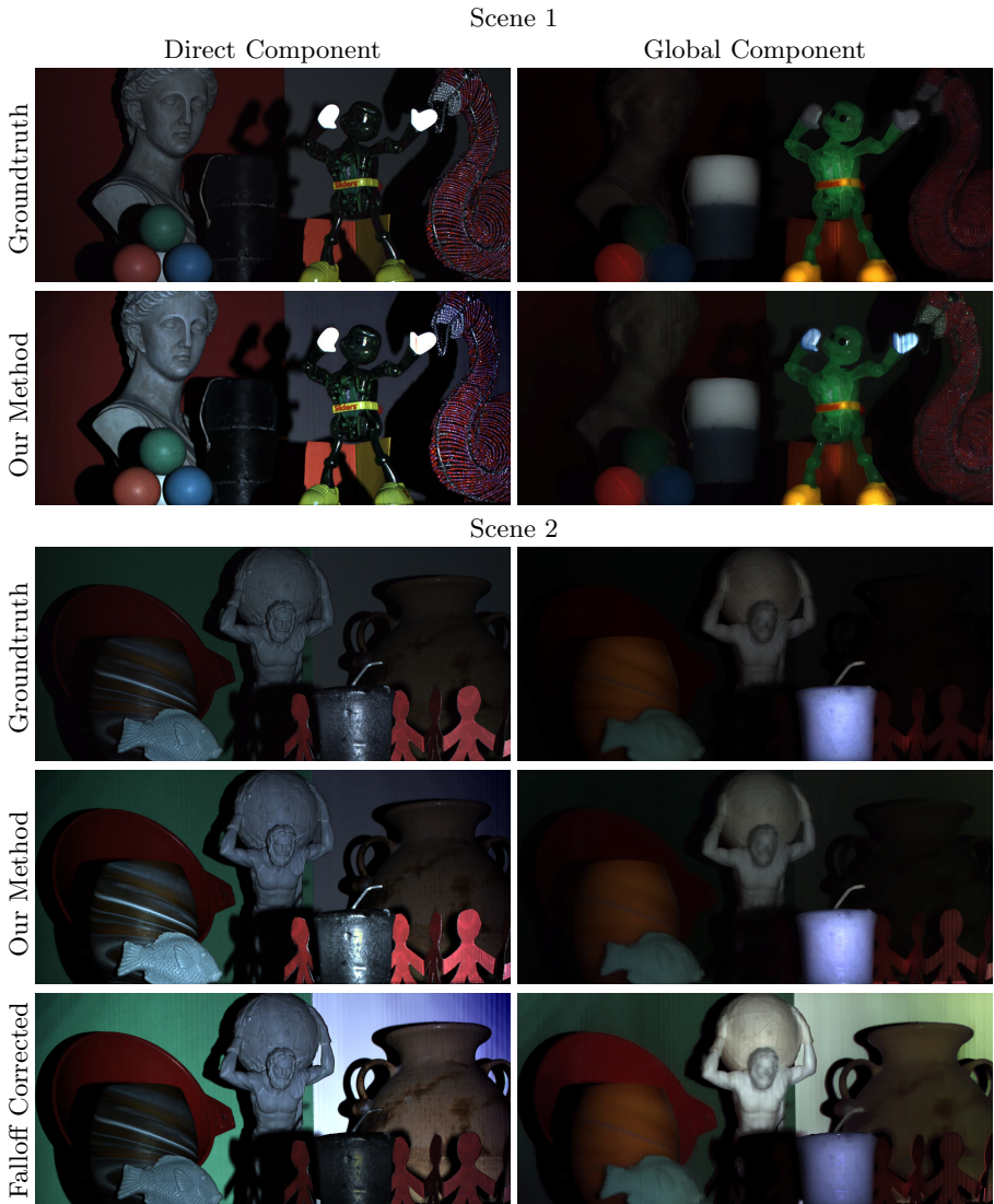
Fig. 8. Direct-Global Separation. Groundtruth was computed using 112 images and our method used 28. In scene 1, the white hands on the robot toy appear much brighter in the global image computed by our method than the ground truth. This is because our algorithm tried to fit a linear trend to saturated (completely white) camera pixels. In scene 2, the shading on the soap fish and the white statue becomes is very clear in the direct illumination image.
