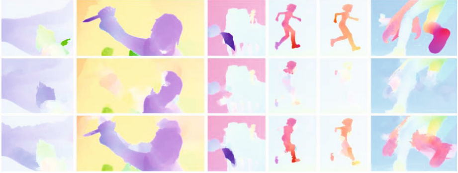
Fig. 7. Details of results on the albedo training sequences. Top row: Ground truth. Middle row: Flow estimation with the traditional approach often fails to capture large motions, especially of smaller objects. Bottom row: Using CR's to represent the image improves the accuracy of the flow in such difficult regions. Some examples are (from left to right): Sintel's hair, the arm and knife, the bat's wing, Sintel's limbs, Sintel's body, Sintel's foot.
