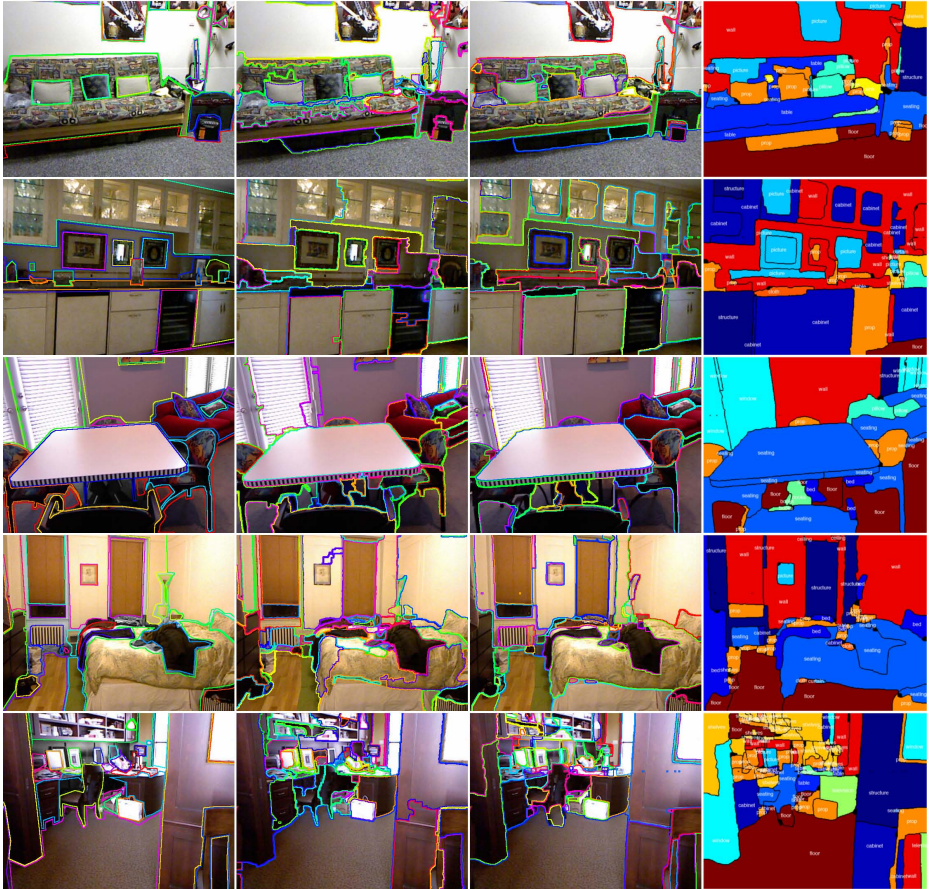
Fig. 3. Random test images from the NYU Depth V2 dataset, overlaid with segmentations. 1st column: ground truth. 2nd column: segmentations from Jia et al [34]. 3rd column: our segmentations. 4th column: semantic labels, produced as a by-product of our segmentation procedure.
