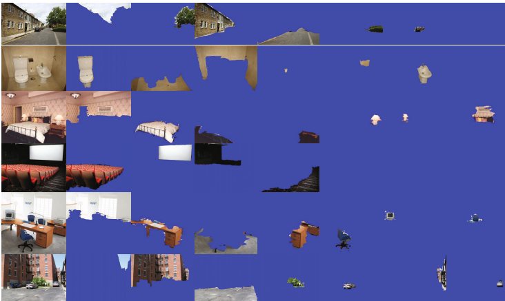
Fig. 5. Scene image co-segmentation examples on LabelMe and SUN. From top to bottom: Outdoor, Bathroom, Bedroom, Movie Theater, Static Office and Static Street. The first column represents an example image, while the rest columns are the results after co-segmentation. The selected segments are ranked in a decreasing order by their overall importance scores from left to right. The blue subgraphs at the tail of each row are only for alignment.
