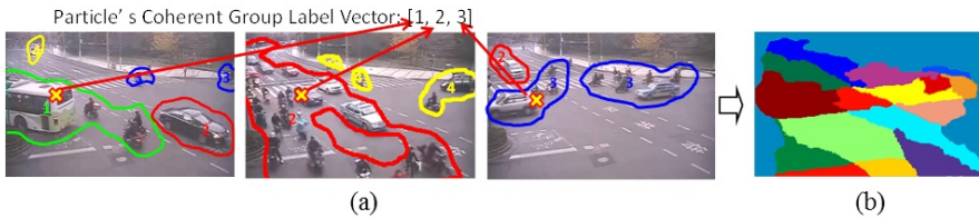
Fig. 5. (a) Step 1: Coherent regions in the three TEFs have been assigned different cluster labels by Step 1 and are displayed in different colors); (b) Find semantic regions by clustering the cluster label vectors of the particles (best viewed in color)
