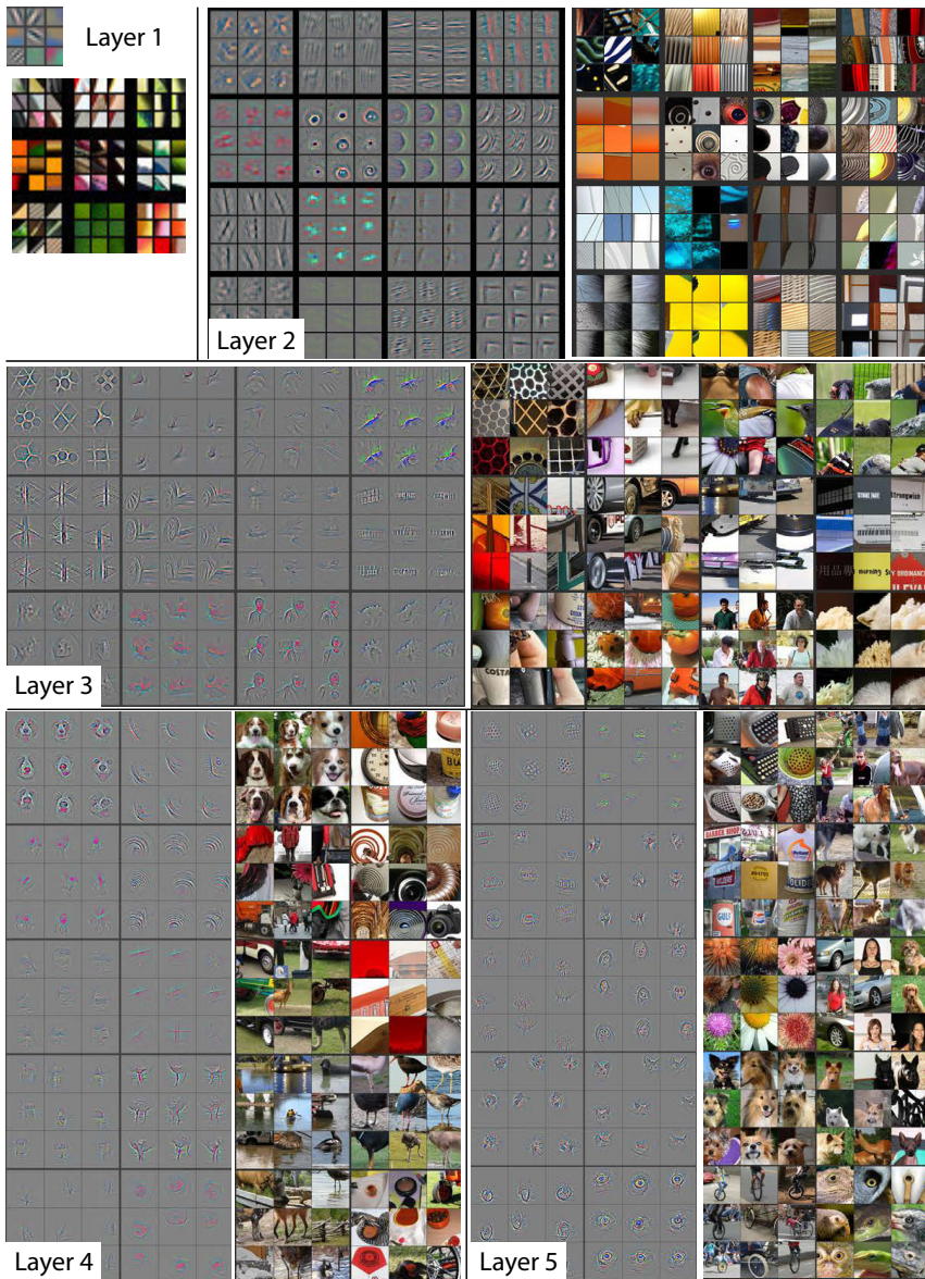
Fig. 2. Visualization of features in a fully trained model. For layers 2-5 we show the top 9 activations in a random subset of feature maps across the validation data, projected down to pixel space using our deconvolutional network approach. Our reconstructions are not samples from the model: they are reconstructed patterns from the validation set that cause high activations in a given feature map. For each feature map we also show the corresponding image patches. Note: (i) the strong grouping within each feature map, (ii) greater invariance at higher layers and (iii) exaggeration of discriminative parts of the image, e.g. eyes and noses of dogs (layer 4, row 1, cols 1). Best viewed in electronic form. The compression artifacts of the 30Mb submission limit, not the reconstruction algorithm itself.
