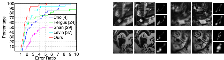
Fig. 6. Left: Error ratio evaluation for the benchmark dataset [24] (evaluation scores for other methods are taken from [23], [24]). Right: A few of our results for the dataset in [24] (for each one we show: input & deblurred images, true & estimated kernels).
