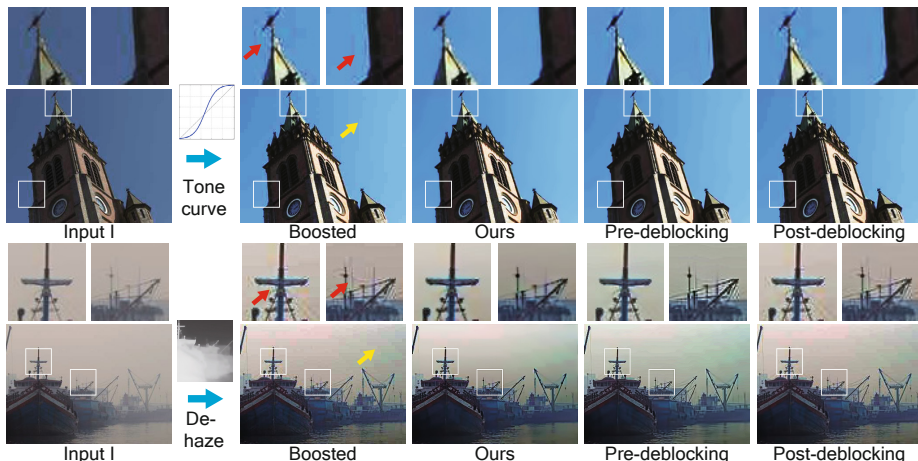
Fig. 1. This shows the noticeable compression artifacts after contrast enhancement. Top two rows are a tone-curve adjustment case ( Q40 ) and the bottom two rows are a dehazing case ( Q70 ). The zoomed-in regions are listed above to show the details. The characteristics of the blocking artifacts are distinctive in smooth regions (pointed out by the yellow arrows), while the ringing artifacts are along strong edges (pointed out by the red arrows). Comparison of our results with those of the deblocking method [10] applied before or after contrast enhancement results are shown. Note, our method produces more compelling results for reducing both blocking and ringing artifacts.
