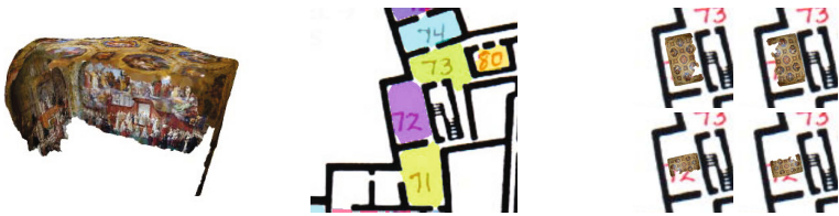
Fig. 3. Left: A 3D piece of our system corresponding to the Hall of the Immaculate Conception. Middle: Colored 2D regions extracted from the floorplan. Number 72 in purple corresponds to the ground truth location of the 3D piece. Right: Candidate placements of the 3D piece to the 2D region.
