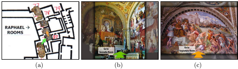
Fig. 9. Screenshots of our interactive visualization: (a) The annotated map is shown with the aligned 3D models rendered on top. When the user clicks on the model of the Hall of Immaculate Conception, the visualization flies into the room showing a photo taken in it (b). An arrow points to the location of the next room, the Incendio Room, and when clicked, the visualization flies the user to that room (c).
