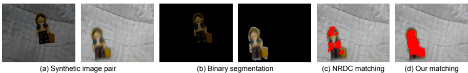
Fig. 8. Differences in correspondence density between our method and NRDC [7]. Our method establishes non-rigid dense correspondence between two segmented region pairs (b). For the motion-blurred object region, (c) shows the matched patches with NRDC, and (d) shows a thresholded version of our transferred matte.
