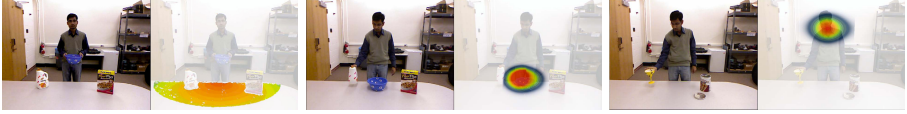
Fig. 5. Distribution over trajectory goal locations. The heatmaps show the distribution over goal locations for placeability (left), pourability (middle) and drinkability (right). The red signifies the most likely goal location for a given affordance.
