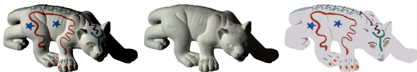
Fig. 1. An example of the intrinsic image problem. Left-to-right: original image, inferred shading and reflectance images under the proposed method.
