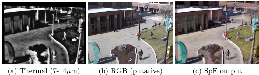
Fig. 6. Example of thermal + RGB fusion; images taken from OTCBVS dataset [9]
