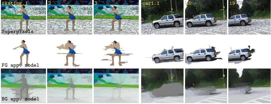
Fig. 6. Visualization of the foreground/background appearance models. Note that the proposed temporal propagation scheme maintains accurate appearance models, even where the background scene is occluded by foreground objects. Gray areas in the images for background appearance denote the absence of appearance models, and our algorithm learns the models quickly using new observations.
