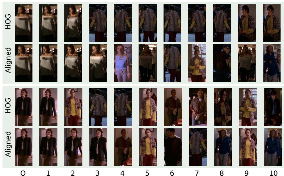
Fig. 3. Nearest neighbor queries showing query image Q and its 10 nearest neighbors. The 1st and 3rd row show the query result using HOG features without alignment. The 2nd and 4th row use alignment energy E as distance and show the nearest neighbors warped to the query image. The alignment based distance returns more similar instances, demonstrating that it is more invariant to deformations than simple HOG based distances.
