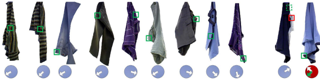
Fig. 7. Success and failure cases (the last two) of some clothes. The arrow under each cloth indicates its pose. The first error is in grasp point detection, the second in pose estimation.
