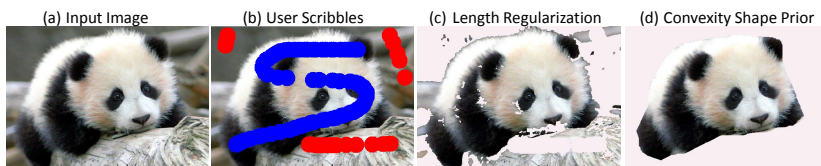
Fig. 1. Segmentation with convexity shape prior: (a) input image, (b) user scribbles, (c) segmentation with contrast sensitive length regularization. We optimized the weight of length with respect to ground truth. (d) segmentation with convexity shape prior.
