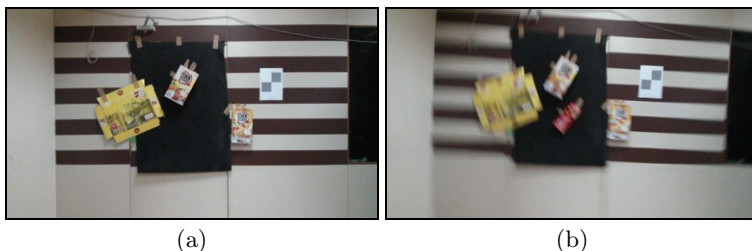
Fig. 1. (a) Reference image with no camera motion, (b) Distorted image with rolling shutter and motion blur artifacts
