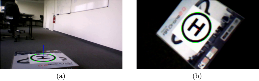
Figure 5. Landpad detection results using the forward-facing camera (a) and the downward-facing camera (b) of the quadrotor with superimposed normals to the supporting plane of the landpad.
