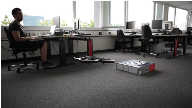
Figure 1. In our method, we detect the circular landpad marker using the forward-facing camera, estimate the distance, and fly towards landing spot by employing monocular SLAM. Once the quadrotor has reached the target position, it tries to detect the landpad using the downward-facing camera, stabilize its position, and finally land.
