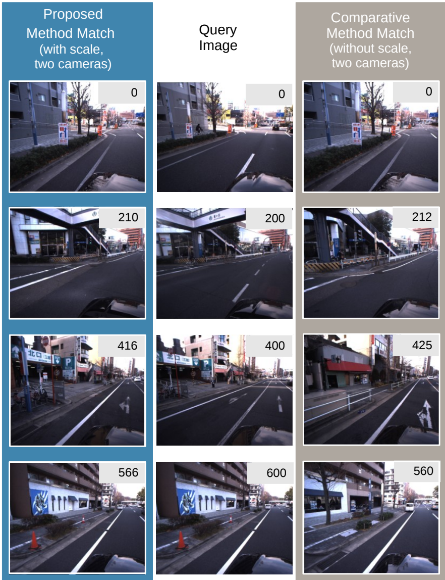
Fig. 4. Sample images showing DTW matching results. The central column is the query image, and the one on left the corresponding matched street map image using the proposed method. The column on the right shows the matched street map images using the comparative method. The numbers in the top right of the images are the sequence frame numbers, showing how DTW matching absorbs differences in vehicle speeds between the visual street map and query image sequences. Note that although results from using both cameras are displayed, only the left-hand camera image is shown for clarity.
