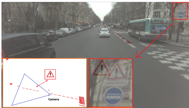
Fig. 1. Projection of 3D road sign and road marking landmarks on an image frame with raw camera pose (Left bottom: camera's field of view shown by blue triangle; middle bottom: zoomed view of the projected 3D road sign on image frame)
