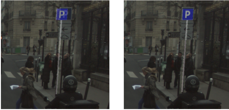
Fig. 7. Segment 1: Left: reference landmark overlapped on image frame with predicted vehicle pose; right: reference landmark overlapped on image frame after vehicle pose correction
