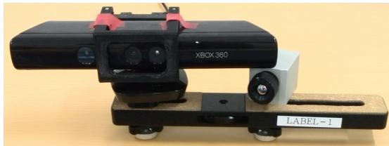
Fig. 1. Our capture system is made of the Microsoft’s KINECT and the optris PI160.
