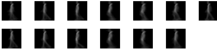
Fig. 5. Thirteen key poses derived for representing a gait cycle
