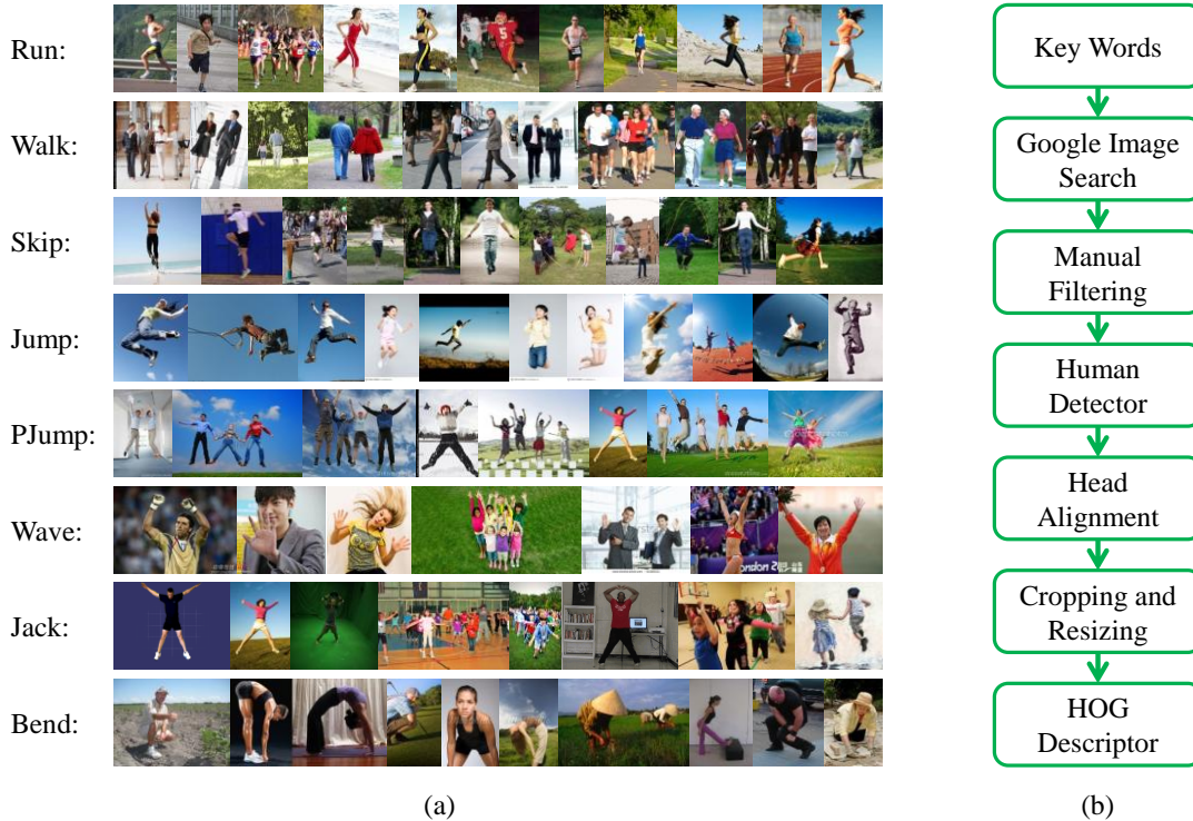
Fig. 1. Examples of web images returned by Google image search, where the action names from top to bottom are ‘run’, ‘walk’, ‘skip’, ‘jump’, ‘pjump’, ‘wave’, ‘jack’, and ‘bend’ (a), and (b) the flow chart of generating the HOG descriptor.
