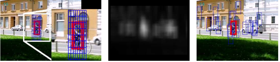
Fig. 1. Illustration of different sampling strategies of negative examples (blue). Left: traditional sampling at fixed positions within a search window around the object (red). Middle: the motion probability density function m (Eq. 11). Right: the proposed negative sampling from m .
