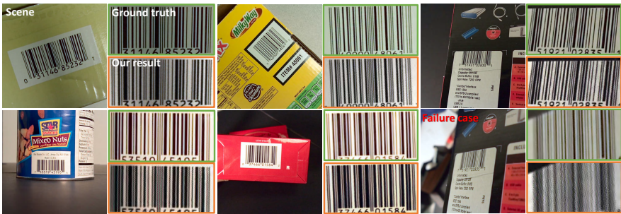
Fig. 9. Rendering results of real barcodes using our scanning system. The full image on the left of each barcode example is the in focus image at the ground truth depth. We also show an example where our algorithm fails due to severe distortion.
