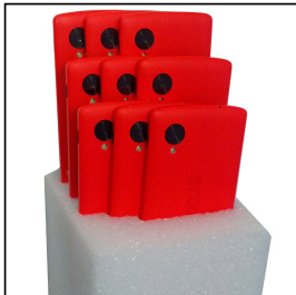
Fig. 5. Camera array setup used for evaluation. (Left) Up to 9 cameras are placed in an rigid array to minimize errors not associated with scene motion. (Right) Camera synchronization timings measured in evaluation for NaiveSync (i.e. timestamp comparison) and SocialSync. SocialSync offers tighter synchronization than NaiveSync
