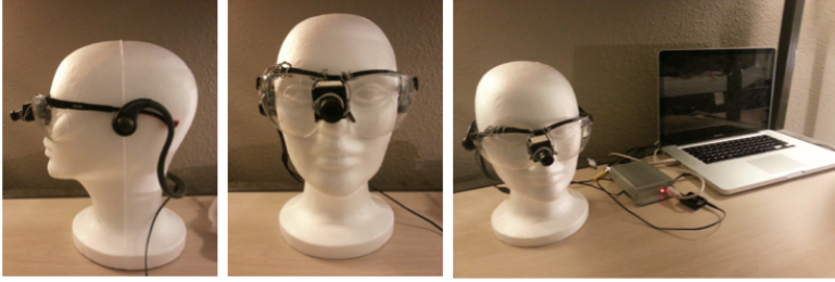
Fig. 4. OLTS hardware. A camera mounted to glasses sends visual input to the computer. The computer houses the vision and feedback algorithms. The bone conduction headphones relay information to the subject.
