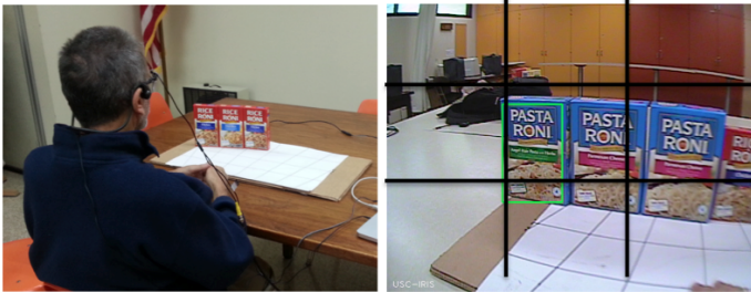
Fig. 8. (Left) Subject wearing the head mounted camera and bone conduction headphones. (Right) Example scene with objects and 9-region grid overlaid.
