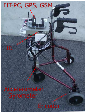
Fig. 1. The instrumented walking aid. Fig. 2. Simple kinematic model of the walker.
