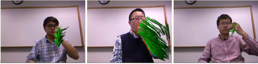
Fig. 6. Position checking is a more subtle action than shaking. The user may slowly or suddenly move the device towards his or her face. As a result, we get trajectories of varying lengths for this action.
