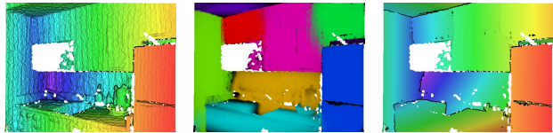
(a) Kinect Depth Map (b) Mixture of Gaussians (c) Plane-Fit Depth Map
