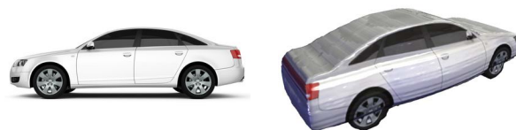
Figure 1. 3D reconstruction result from the single car image on the left based on relative volume constraints. Given a 2D image we infer the object geometry based on shape profiles and volume ratio constraints. These are either imposed by the user or estimated from shading information.
