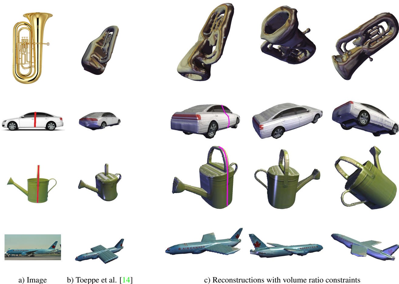
Figure 7. 3D reconstruction results a) without further constraints [14] and b) with application of volume ratio constraints. Relative depth profiles are marked in red (location) and pink (depth function).
