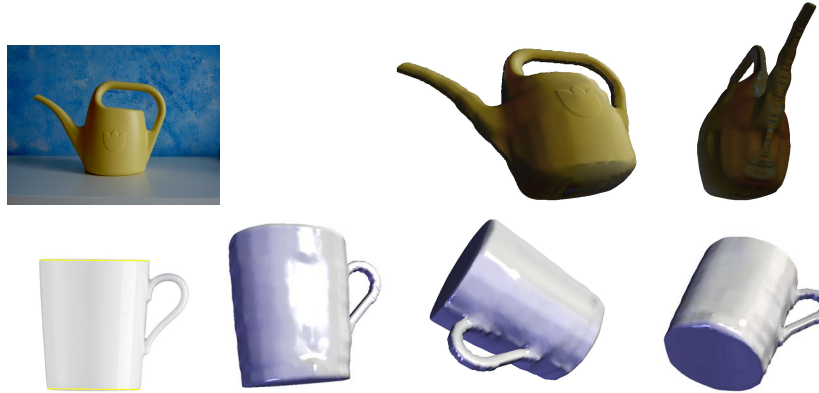
Figure 6. 3D reconstruction results with automatically estimated depth profiles based on shading information.
