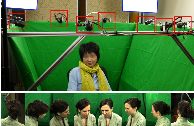
Figure 3: Our hair capture setup and a few sample images. We use 8 cameras (outlined in red) in wide-baseline to capture the complete hair styles. Four area lamps (outlined in blue) are used to compensate for the short exposure time.
