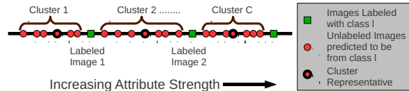
Figure 1: Our clustering approach for fast active learning. Unlabeled images are clustered along each relative attribute using boundaries marked by labeled images of each class. A ranking function is trained for each cluster representative instead of each unlabeled image.
