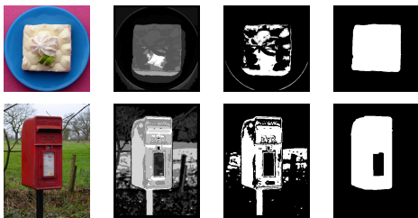
Figure 7: GrabCut segmentation [23] based on statistical textural distinctiveness. From left to right: Input image, saliency map computed with our approach, segmented image after adaptive thresholding, and GrabCut segmentation.
