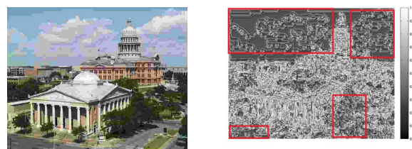
Figure 6. Left: JPEG distorted image from the LIVE database; Right: the local quality map predicted by the proposed QAC method. The areas highlighted by red rectangles are of the worst quality, which are identical to human perception.
