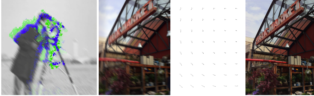
Figure 1. Left: Snapshot of the algorithm in progress showing stochastic random walks that form the basis of Stochastic Deconvolution. Green points represent energy added while blue correspond to energy subtracted from the reconstruction. The algorithm automatically focuses sampling effort in regions where the largest improvements to the system energy are obtained. Right: Example of deblurring with a spatially-varying (per-pixel) PSF simulating strong motion-blur. Input image (center-left) and a sampling of per-pixel PSFs at full-scale (center-right). Deblurred result using Stochastic Deconvolution algorithm (right). The Stochastic Deconvolution algorithm naturally handles PSFs with strong spatial variation, including rotations around the optical axis, without resorting to patch-based approximations.
