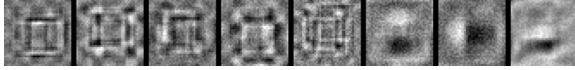
Figure 7. Eight feature detectors of an MLP trained to remove a square blur. The MLP was trained on the blurry patches themselves ( i.e. no pre-processing). The features are large compared to the output patches because the information in the input is very spread out, due to the blur.
