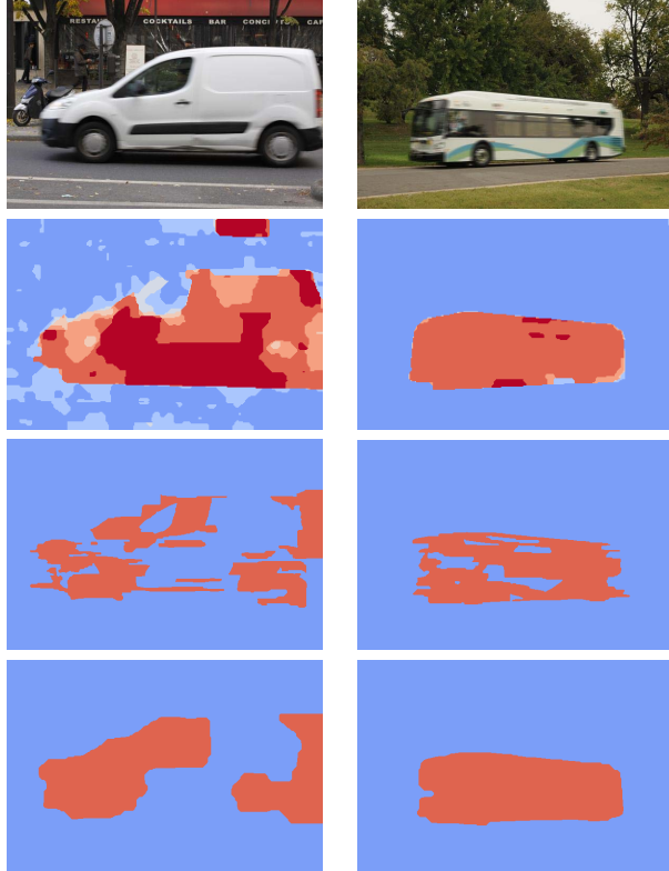
Figure 4. Blur estimation for real (left) and synthetic (right) images with horizontal motion blur. From top to bottom: input image, estimated blur (regions shown in red) with unary and binary costs, the result of [5] using only blur cues, and [5] with blur as well as object cues. We observe that our approach better handles texture-less regions.
