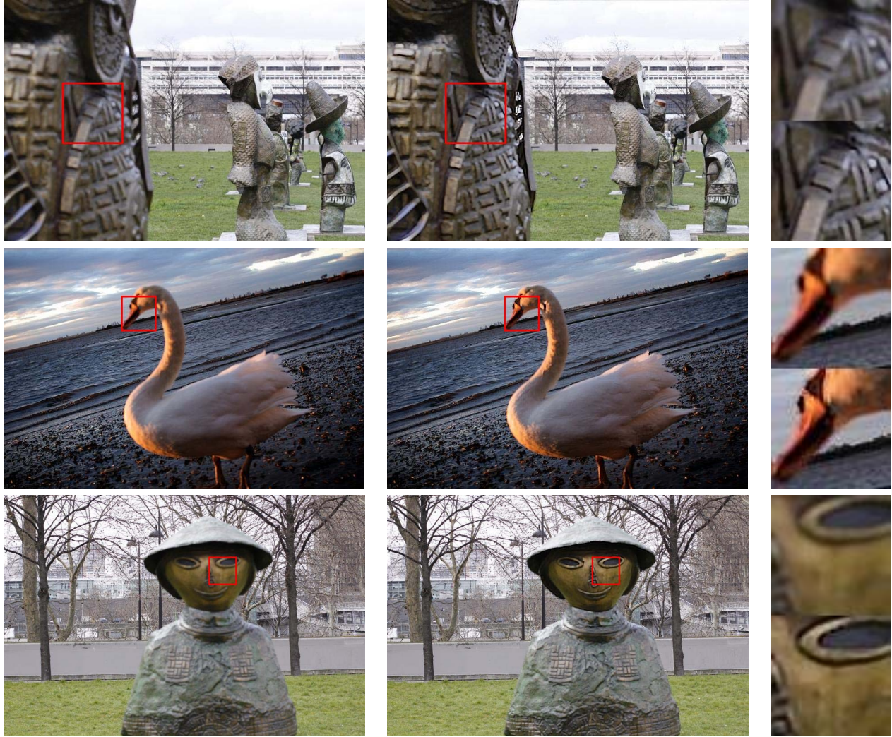
Figure 8. Defocus blur: Sample deblurring results on real images. From left to right: blurry image, deblurred image, close-up corresponding to the boxes shown in red. Note that our estimated deblurred image has more detail. ( Best viewed in pdf. )
