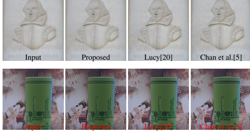
Figure 7. Result of optical defocus deblurring using real camera sensor data with (top row) global and (bottom row) varying depth. Although methods in [5, 20] cannot handle non-global blur, top row is a fair comparison of the reconstruction quality, while the bottom row shows a more realistic scenario. The bottom row was rendered with background blur for [5, 20] and using Figure 6(b) for the proposed deblurring method.
