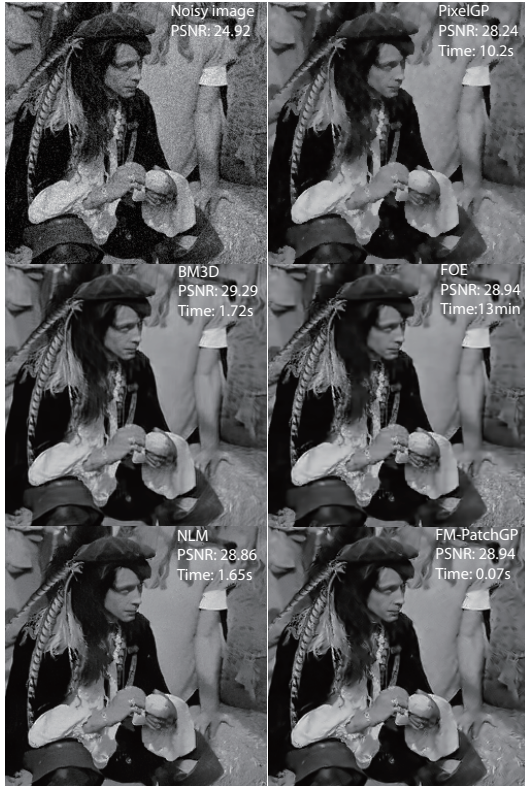
Figure 6. Denoising results on the ‘man’ image with Gaussian noise \sigma_n = 15 . Our result is comparable state-of-the-art but is one to three orders of magnitude faster.
