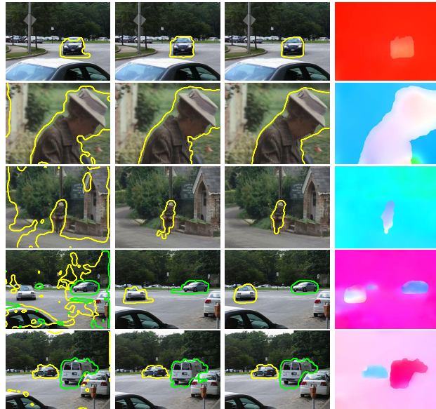
Figure 9. Results of global-local algorithm (third column) in motion segmentation in comparison to fully global (left column), and fully local algorithms (second column). The fourth column is the optical flow field determined by the global-local algorithm (using the standard color scheme). The global-local tradeoff algorithm avoids clutter, and is less susceptible to irrelevant fine detail.
