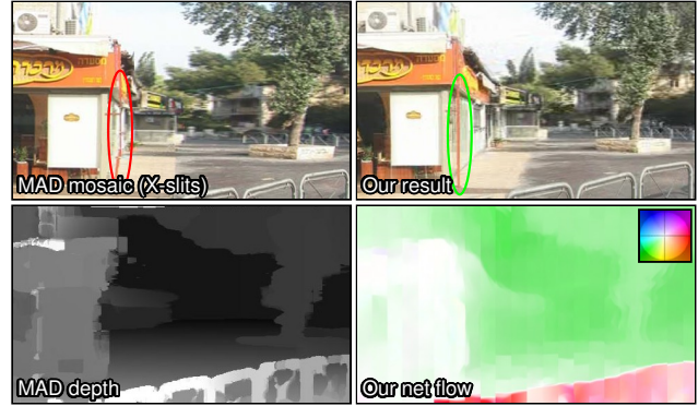
Figure 9. Our flow-based blending compared to the depth-based stitching of Rav-Acha et al. [16] on their dataset ‘refaim’.
