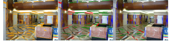
(b) Our algorithm detected 2 orthogonal triplets (middle and right), and assigned the blue direction as being common for both.
