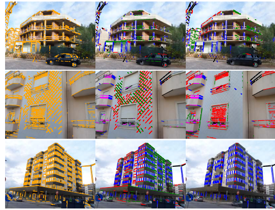
Figure 9. (Left) extracted edges, and (right) detection results. In each example (row) we detected 2 groups of orthogonal triplets with the blue VD in common. The VD in magenta (row 3) was detected but (incorrectly) not assigned to any triplet.
